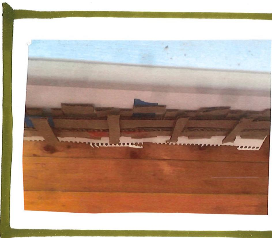
This prototype gave me a look at a 3d design of the fence and what it was going to look like. This prototype was successful as it showed me that the design could be stable once the post are put into the design.
